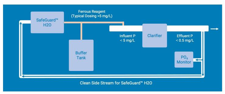
Figure 1. SafeGuard™ H2O Phosphate Removal Process
