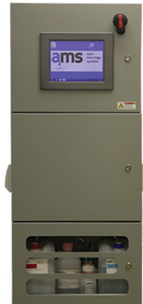
MetalGuard™ Iron is a fully automated, online iron analyzer.
