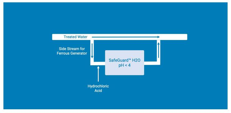
SafeGuard<sup>™</sup> H2O Arsenic Removal Technology Schematic
