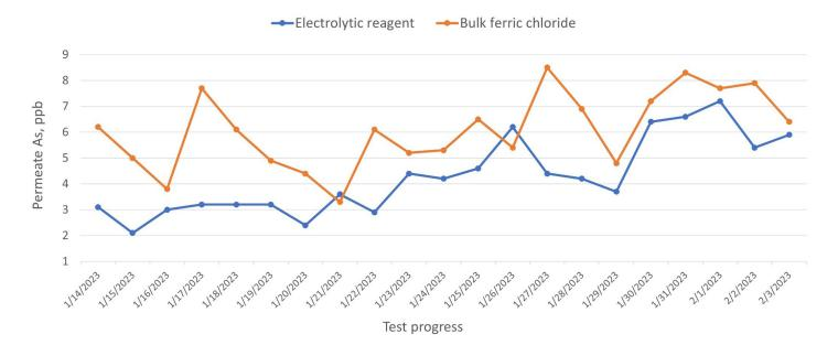
Total Arsenic in Train 1 (Bulk Ferric Chloride) and Train 2 (Electrolytic Ferrous Reagent) Permeates
