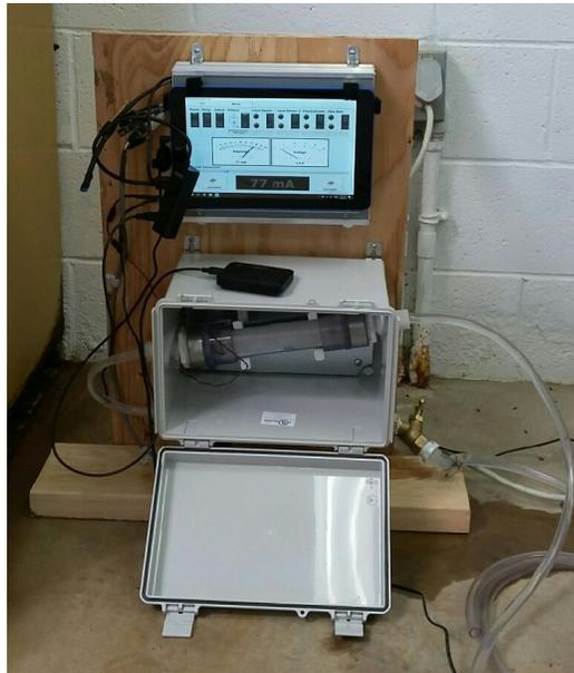
**Figure 1: SafeGuard™ H2O Online Cr(VI) Remediation System Demonstration Unit**
